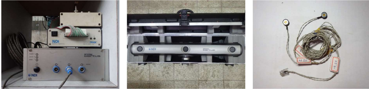
Figure 2. The optical measuring system: (a) controller, (b) camera, and (c) marker.
