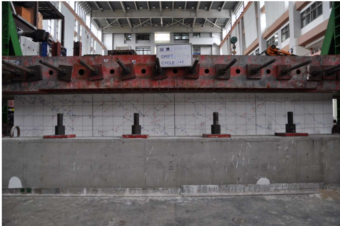
圖 23 試體 EFB-48 強度點正面照(Drift Ratio = 0.3%)[左側為西]
